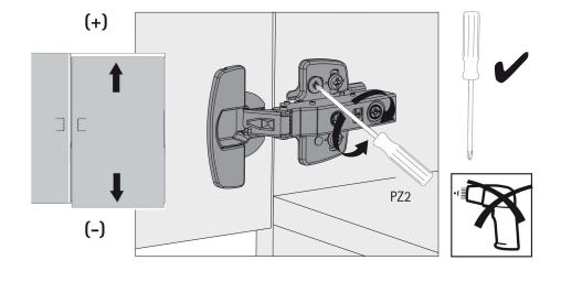
Height adjustable mounting plates permit exact alignment of door. Direct, infinitely variable height adjustment by eccentric screw.
