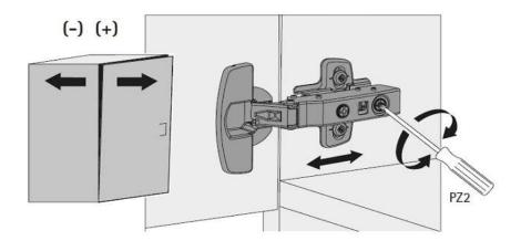
Direct, infinitely variable depth adjustment.
